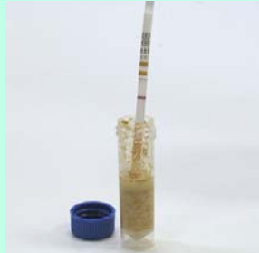
Place strip in extraction vial
